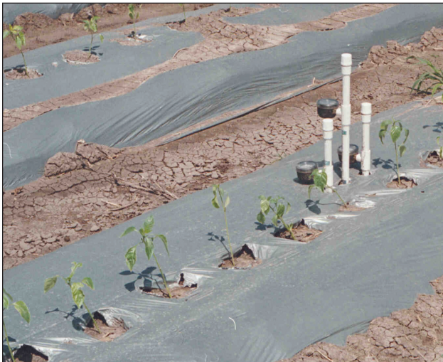
Fig. 11. Station of 3 tensiometers installed at different soil depths.
