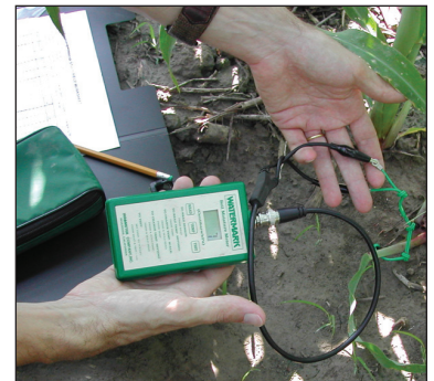
Figure 4. Using handheld meter for Watermark® sensor.
