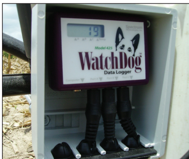
Figure 5. Watermark® sensors connected to a 3-port WatchDog® data logger.
