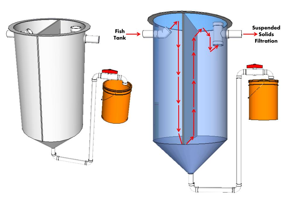
Clarifier Tank Settleable Solids Removal
